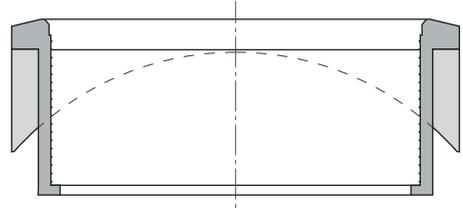
The Tubocor seal withstands a water pressure of 0,5 bar
